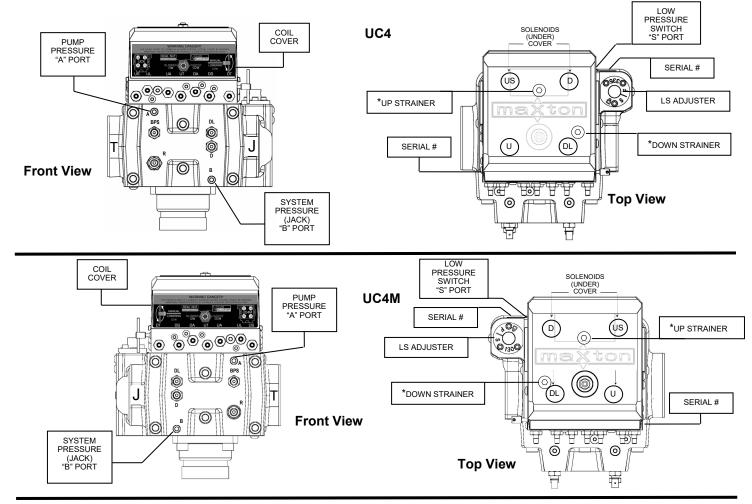
**ATTENTION:** All Maxton Valves **MUST** be installed with the solenoids in the upright (vertical) position. When replacing a Maxton UC3 / UC3AM or UC4 / UC4M series valve, the pump flange assembly must also be replaced. It is subject to the same wear and tear as the valve. \*Strainer access is provided from the top of the control plate. Prior to 2012 the sleeve and baseplate were an integral part of coil operation. 2012 to current the C-Frame is an integral part of coil operation.
