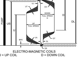
CAUTION: On Wye - Delta Up Start do not energize U and US Coils until motor is running on Delta. With soft starter, energize US coil with motor up to speed signal.
