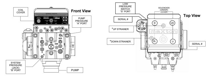
\* Strainer access is provided from the top of the control plate. Prior to 2012 the sleeve and baseplate were an integral part of coil operation. 2012 to current the C-Frame is an integral part of coil operation.
