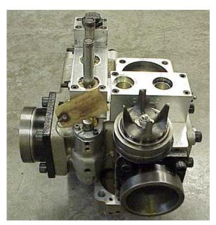
In an effort to drastically reduce costs some repair facilities will re-use scrap obsolete parts when repairing your elevator control valves.
