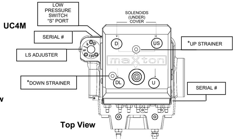
**ATTENTION:** All Maxton Valves **MUST** be installed with the solenoids in the upright (vertical) position. When replacing a Maxton UC3 / UC3AM or UC4 / UC4M series valve, the pump flange assembly must also be replaced. It is subject to the same wear and tear as the valve. \*Strainer access is provided from the top of the control plate. Prior to 2012 the sleeve and baseplate were an integral part of coil operation. 2012 to current the C-Frame is an integral part of coil operation.
