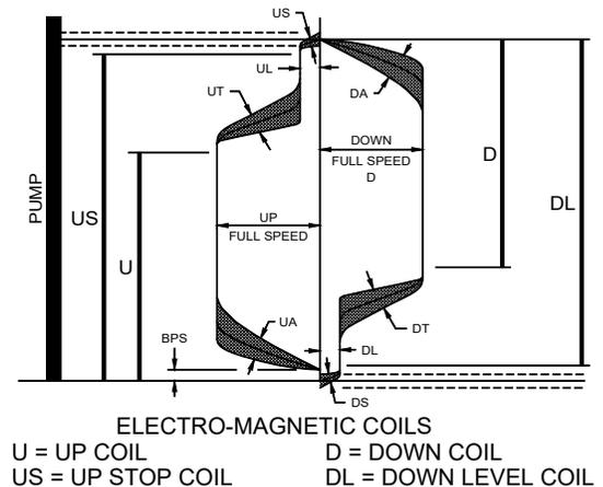
**CAUTION:** On Wye - Delta Up Start do not energize U and US Coils until motor is running on Delta. With soft starter, energize US coil with motor up to speed signal.
