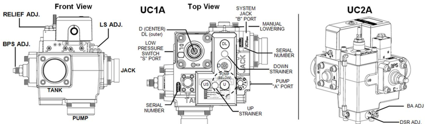
**ATTENTION:** All Maxton Valves **MUST** be installed with the solenoids in the upright (vertical position). Prior to 2012 the sleeve and baseplate were an integral part of coil operation. 2012 to current the C-Frame is an integral part of coil operation.
