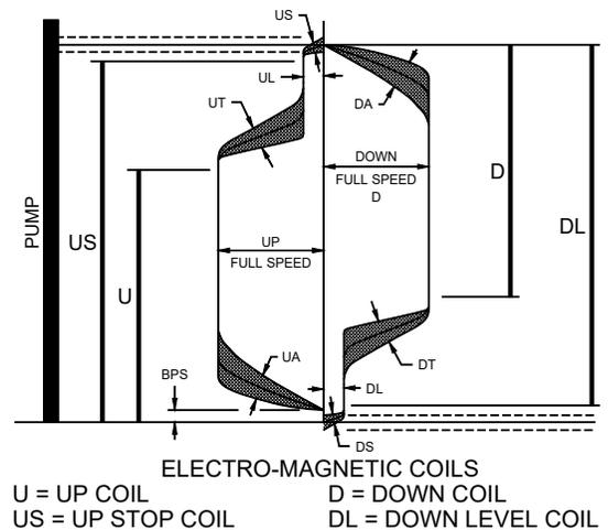
**CAUTION:** On Wye - Delta Up Start do not energize U and US Coils until motor is running on Delta. With soft starter, energized US coil with motor up to speed signal.
