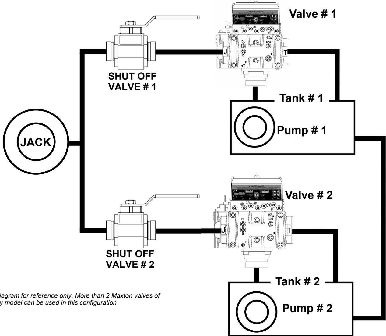
*\*Diagram for reference only. More than 2 Maxton valves of any model can be used in this configuration*
